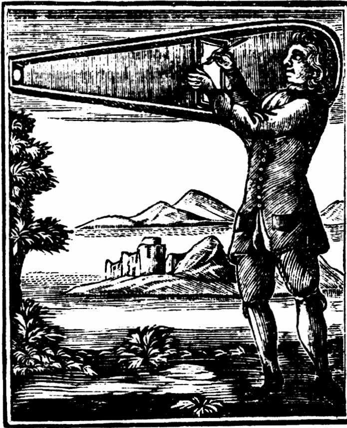
Abb. 1. Tragbare Camera obscura ( picture-box ) als Zeicheninstrument. Holzschnitt von 1694 in: Robert Hooke: An Instrument of Use to take the Draught, or Picture of any Thing . Communicated by Dr. Hooke to the Royal Society Dec. 19, 1694, in: Philosophical Experiments and Observations of the late Eminent Dr. Hooke [...], ed. by William Derham, London 1726, S. 295.
