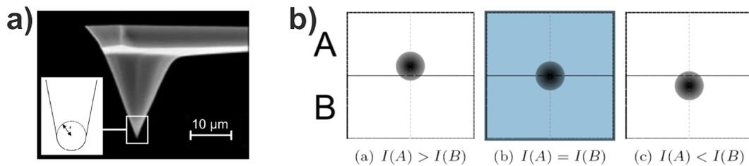
**Abbildung 2:** a) Typical measuring tip; b) Scheme for detecting the position of the laser on a (here two-part) photodiode by a change in the ratio of the intensities measured in areas A and B.
