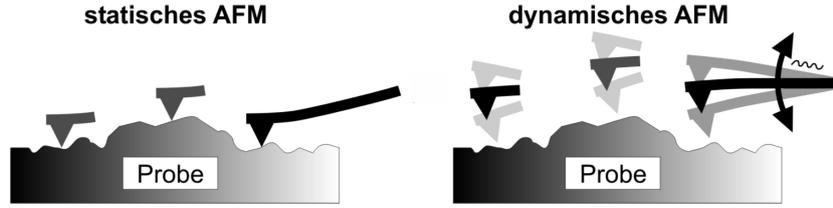
Abbildung 3: Sketch of the function of the static and dynamic mode.
