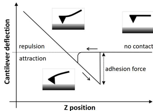
**Abbildung 6:** „Raw data“ of a force-distance curve: The force can be calculated from the bending of the cantilever (knowing its spring constants) and the distance traveled can be calculated from the vertical z-position of the cantilever.
