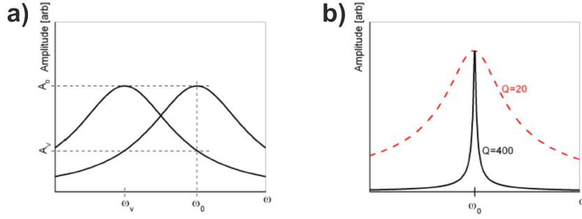
**Abbildung 5:** Oscillation amplitude as a function of frequency  $\omega$ : a) Change in oscillation amplitude (from  $A_0$  to  $A_v$ ) due to a shift in resonance frequency ((from  $\omega_0$  to  $\omega_v$ ). b) Effects of different quality factors  $Q$  on the width of the resonance peak.
