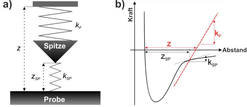
**Abbildung 4:** a) Model of a measuring tip in an interaction potential: The tip is located on a cantilever with a spring constant  $k_F$  and the force of the interaction between tip and sample is assumed to be another spring with a distance-dependent spring constant  $k_{SP}(z_{SP})$ . b) Typical force-distance curve (black) superimposed with the force-bending curve of the cantilever (red) at a distance  $z$  from the surface. (For details on force-distance curves, see section 2.2).
