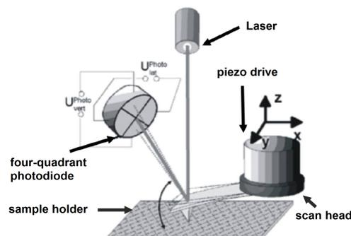
Abbildung 1: Schematic setup of an atomic force microscope.
